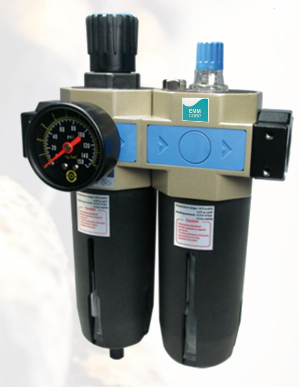
The air line lubricator must be installed no more than 3m from the hoist and should be set to deliver a minimum of 1 to 3 drops per minute when the hoist is running at full speed. The recommended lubricant is a light oil i.e. ISO VG10. Do not use automotive type detergent oil as these oils will delaminate the motor vanes and cause motor failure. The air supply must be shut off before filling airline lubricator.
