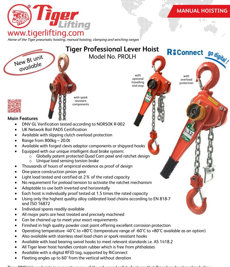
Tiger PROLH lever hoists incorporate many of the advanced safety features that Tiger has developed including one-piece construction pinion gears, our unique intelligent dual brake system and our patented Quad Cam Pawl System. These units meet and exceed all the requirements within BS EN 13157: 2004+A1:2009, ANSI/ASME B30.21, AS1418.2 and SANS 1636.
