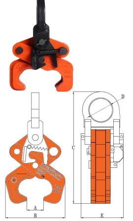
The Tiger CRT rail clamps are designed to lift single rails lengthways and crossways, securely and safely. The clamps are designed to fit most types of rail section currently in use. The clamps are locked onto the rail-head via a lever operated spring mechanism. Very solid, practical design with low dead weight. For rail sizes S49, S54, S60s, UIC60.
